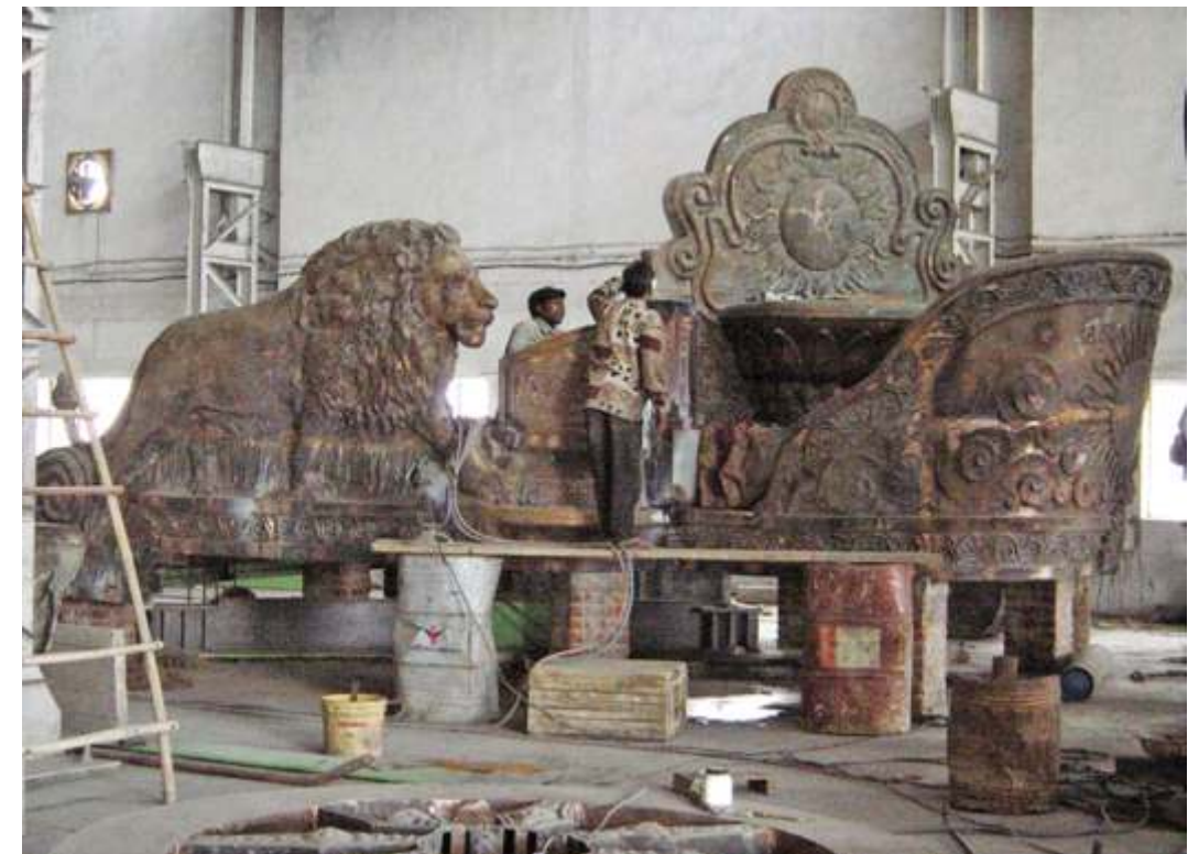
Assembling Bronze parts of Krishna-Arjun Chariot in foundry
