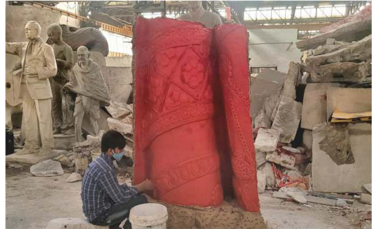
Lost wax process being used to get high quality details in bronze statue
