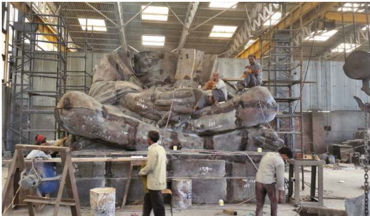
Assembling of Bronze panels in our foundry
